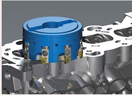
Top Face(Roughing & Finishing) - Aero Mill • Due to the light weight of aluminum body that about 50% of steel body, excellent cutting performance with high speed machining can be achieved.
